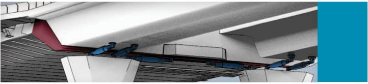
Between each section of bridge road deck are expansion joints and hinges, allowing each section to move without damaging its adjoining sections during an earthquake.
