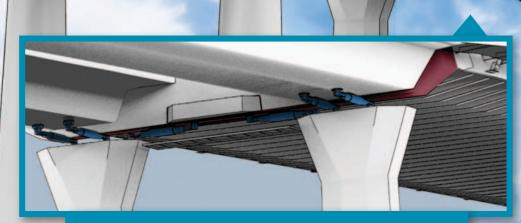
Expansion Joints & Dampers: Specially designed expansion joints and dampers will enable controlled-swivel movements in three directions – vertical, longitudinal, and lateral – to enable flexibility between the column-supported approaches and the cable-supported main span.
